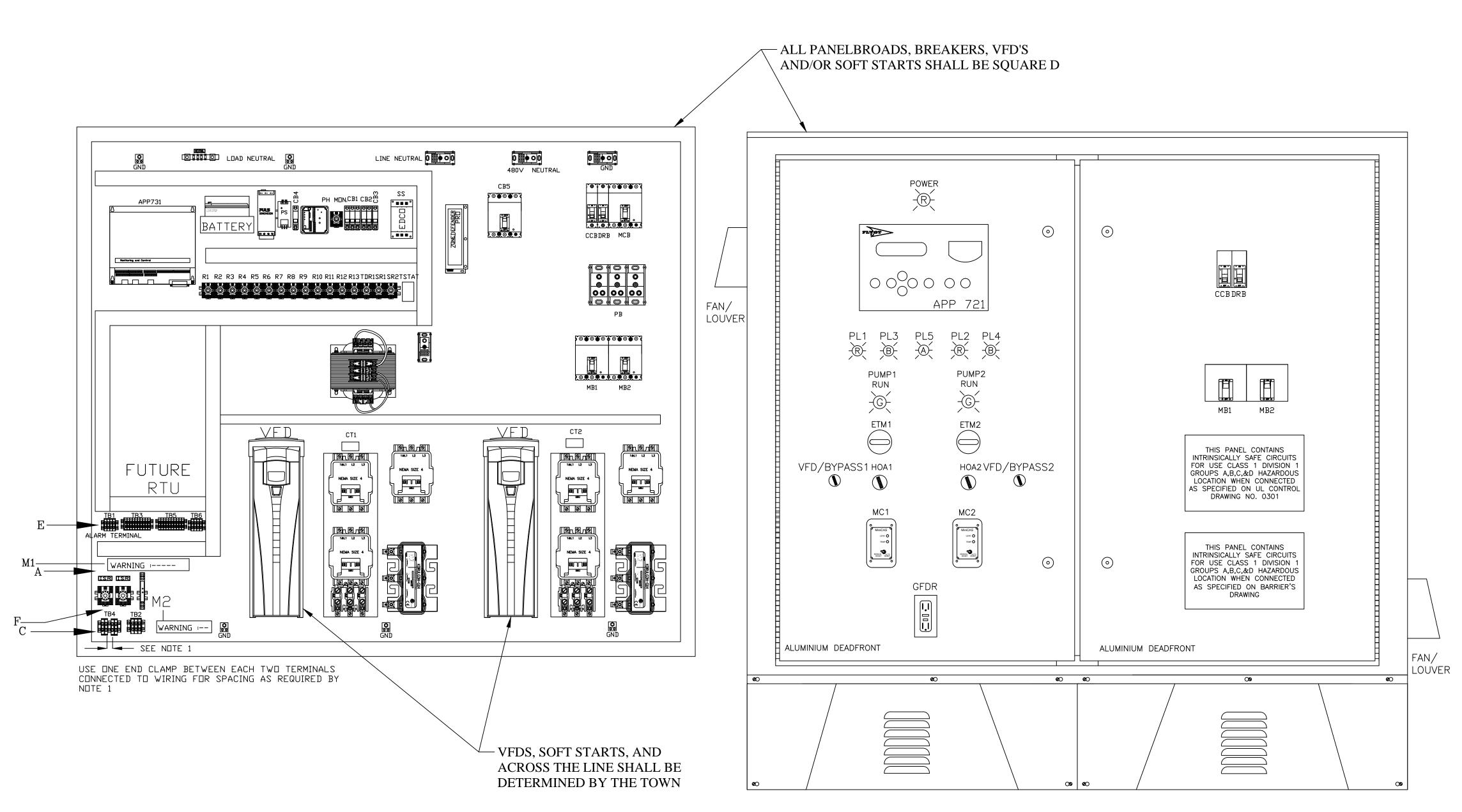
NEMA TYPE 12 P.S. 12GA ENCLOSURE WITH CONTINUOUS HINGES 3 POINT LATCH, PADLOCKABLE (TYPICAL) ACTUAL LAYOUT MAY VARY WITH HORSEPOWER DIMENSIONS: 60" H X 72" W X 14" D 12 INCH LEGS
